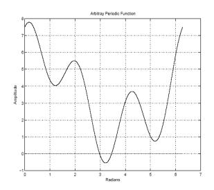
\*\*\*\*\* **Insert Figure 1.9 here**\*\*\*\* Figure 1.9.Addition of constant value of 3.5 shifts the wave to the upper half of axis.
