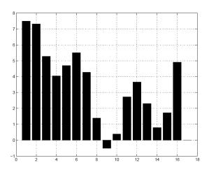
\*\*\*\*\* **Insert Figure 1.12 here**\*\*\*\* Fig 1.12. Integrating the function using rectangular area method
