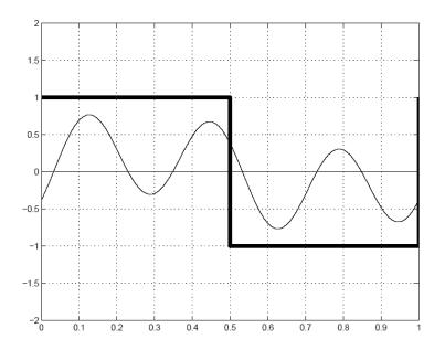
\*\*\*\*\* **Insert Figure 1.14 here**\*\*\*\* Fig 1.14. Response to step function input for the Example 1.2
