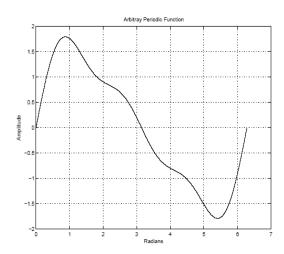
\*\*\*\*\* **Insert Figure 1.7 here**\*\*\*\* Figure 1.7.An arbitrary waveform created by summing up sin functions
